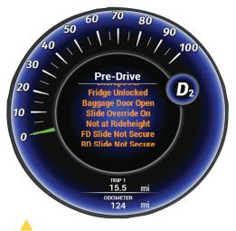
Pre-drive checklist lets you know when it's safe to drive. This display is completely configurable.
