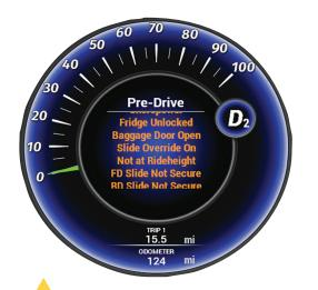
Pre-drive checklist lets you know when it's safe to drive. This display is completely configurable.
