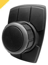
Multiple input options include rotary knob/joystick (left), touchscreen, steering wheel paddles and buttons.
