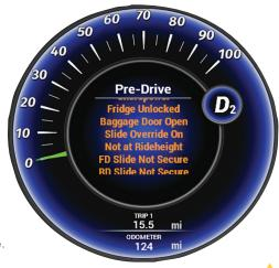
Pre-drive checklist lets you know when it's safe to drive. This display is completely configurable.
